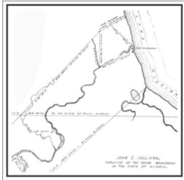
The sketch shows how John C. Sullivan positioned the Indian Boundary Lines 10 miles north and 10 miles south of the mouth of the Chicago River.
